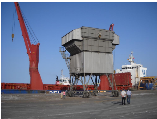
Shipment supervision of a large hopper for bulk cargoes in the port of Huelva (Spain)
